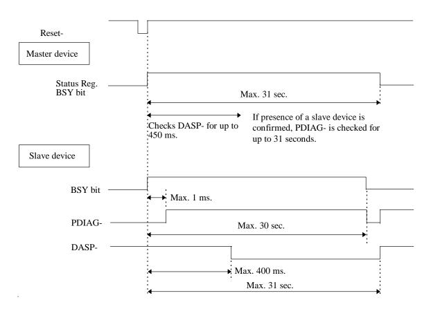
Figure 6.2 Response to hardware reset
